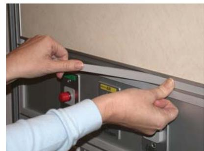
Reinstall the lower fascia and fasten with the six #6-32 screws.
